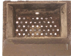
Fire pot needing cleaning with the holes blocked by ashes
